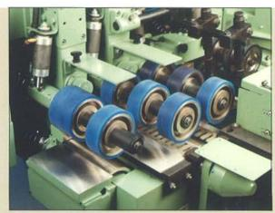
Outfeed Features: 220mm wide outfeed driven bed roller. 50mm staggered side heads. Hydraulically clamped outboard bearings.
